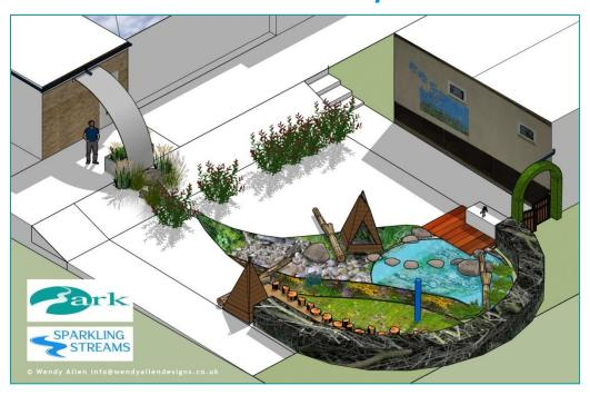
Rain Gardens are uniquely designed gardens that reduce and slow down the flow of storm water into the sewer system.
